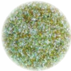
Grade 1 0.5 – 1.0mm (equivalent to Grade 16/30 sand)
