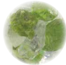
Grade 3 3.0 – 6.0mm (equivalent to Pea Gravel)
